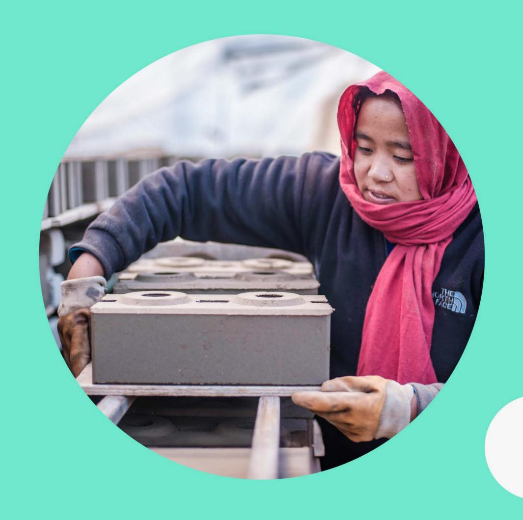
Made from **local materials** like stone dust, the eco-bricks are much cheaper than fired bricks.
